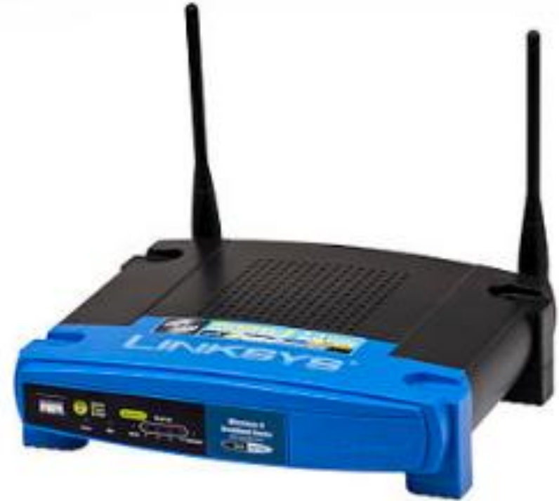
This Linksys WRT54GS WiFi router from 2005 operates on the 2.4 GHz "G" standard, capable of transmitting 54 megabits per second.
