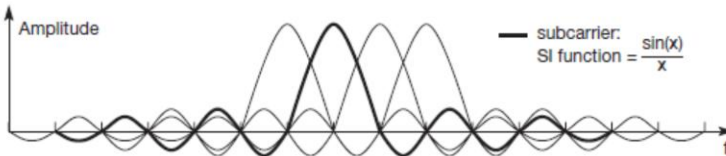
Figure 2.31 Superposition of orthogonal frequencies
