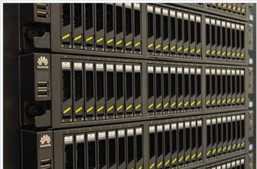
Storage servers housing 24 SAS hard disk drives per server
